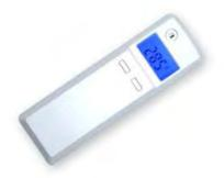
Z716 is a temperature and humidity display. The data can be sent to a data center wirelessly.
